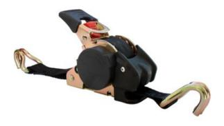
Rollo mini is a lashing for securing lighter cargo. Rollo mini is easy to use and the functionality is like a retractable seat belt. The lashing is rolled out to desired length and then tightened like an ordinary lashing. After usage the band retracts automatically. The lashing only consists of one part which benefits ease of use and simplicity.
