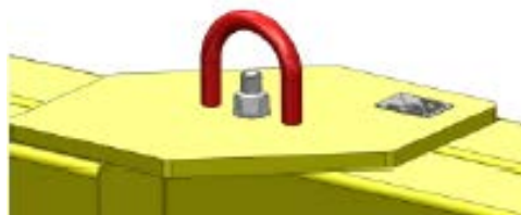
Figure 2: Central lifting point
